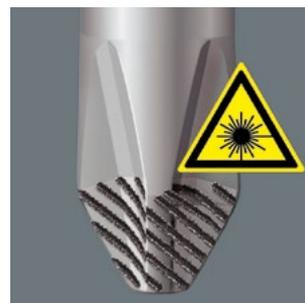
A precisely-focused laser creates a sharp-edged surface structure. This laser treatment results in an edge hardness of up to 1000 HV 0.3. Wera Lasertip “bites” itself into the screw head and prevents any slips out of the recess.
