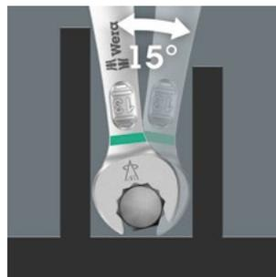
The Joker 6003 ring spanner with its special mouth geometry – mouth side pivoted by 7.5° and the double hexagon profile – doubles the placement possibilities when repeatedly turning the wrench 180° around the longitudinal axis. Bolts and screw heads can be "accessed" every 15°. The
