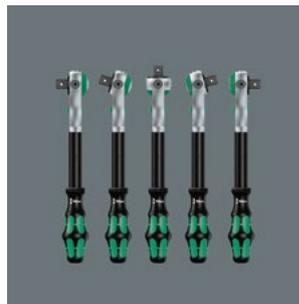
The ratchet head of the Zyklop Speed pivots freely and can be locked into any defined position by using the slide switch that is positioned on either side. It is even possible to work in very confined and difficult-to-access areas with enhanced hand clearance. The predefined locking at 0°, 15° and 90°,
